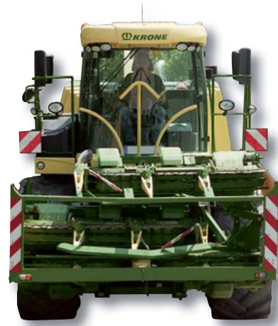
Compact transport width: The three-section EasyCollect model
