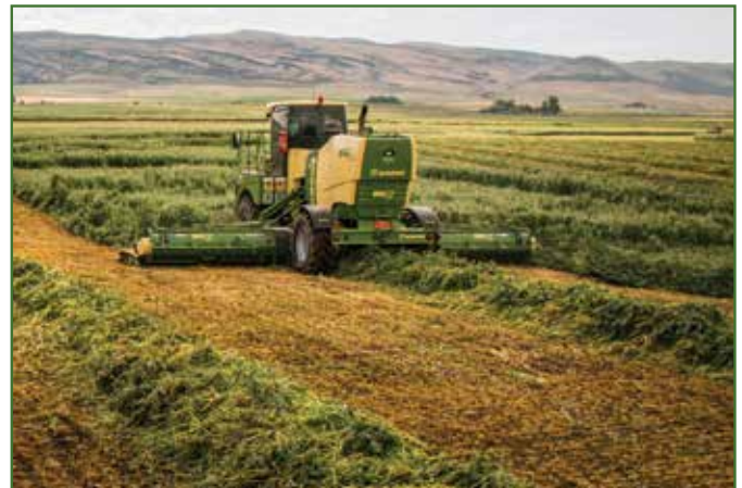
The mergers give users flexibility to merge the crop or lay it flat. This feature is fully controlled from the cab.
