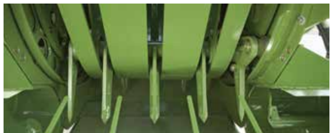
The VFS from Krone produces rock solid, well-shaped bales, no matter the condition. This system operates with four packer rakes and one feeder rake, as well as a retainer. It feeds the material into the pre-compression chamber where it builds a flake. After this pre-compression chamber is packed with material, the feeder rake feeds the material into the baling chamber.
