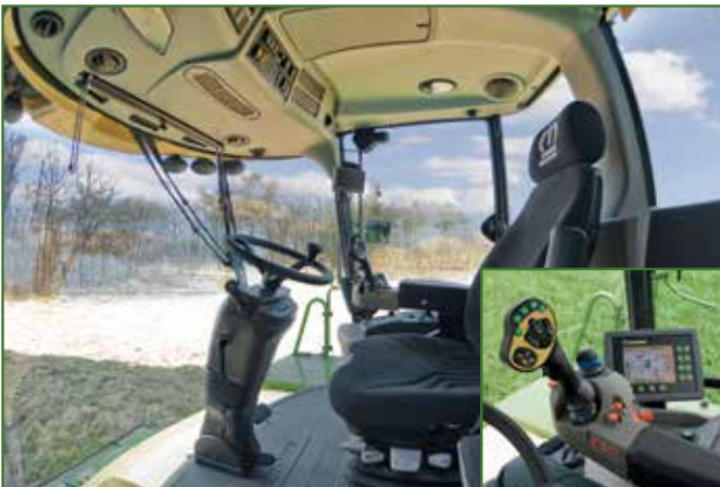
The Krone BiG M cab, with tinted windows and slim posts, offers a perfect view of all mowers. Also, its double floor leads to a significant reduction in noise. Powerful H3 work lights turn night into day.
