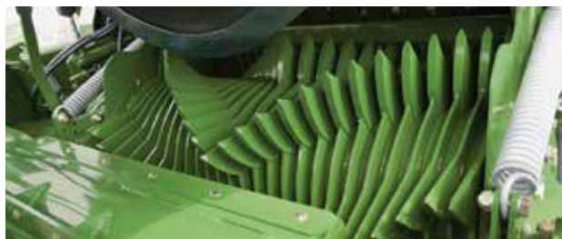
MaxFlow inside: The cut and feed rotor with wide feeding plates are made from hardened steel to enhance the crop flow, while keeping input power low.
